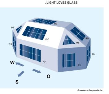
When a PV module is partly shaded, it can lose a significant amount of power. All other modules connected in series within the same circuit will also be affected and will be reduced to the same low power output level as the shaded module. Therefore, shading of the OKACELL element should be avoided as far as possible. Potential casters of shadow can include:
