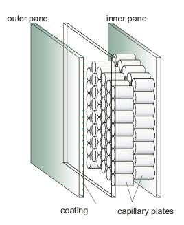
The 2-pane make-up consists of one 20 mm cavity with two 10 mm capillary slabs and covering pane, in general without coating.
