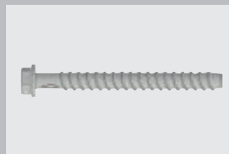
Fischer concrete screw ULTRACUT FBS-II-A4-12 Drilled hole nominal diameter: diameter 12 Aluminium bored hole diameter 15 socket SW 17
