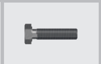
Hex head set screw M 7x28 A4-80 (Flat system screw) Aluminium bored hole diameter 7.5 socket SW 11
